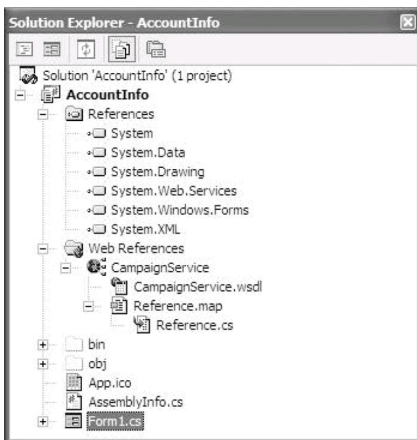
Figure 15-4. You can see the web reference files in Solution Explorer, including the Reference.cs file containing the actual proxy class code
